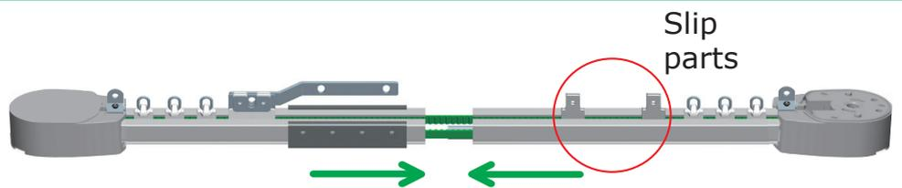
**3** Push the connection bracket into Slip parts.
