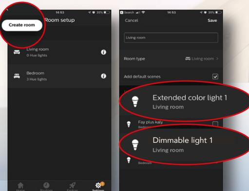
\*If this fails, reset the controller by switching it on and off 5 times. Led strip will blink and glow softly. Repeat steps 1-5.
