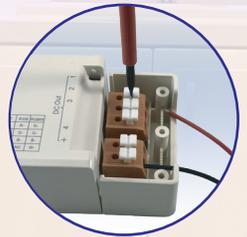
**3** Release the screw driver. Tug gently on the wire to make sure the wire is secured.
