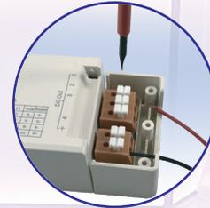
**2** Keep it pushed down and insert the wire.
